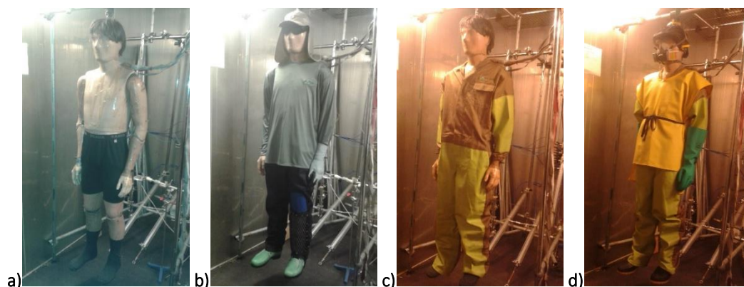
Figure 1: Tested clothing: a) underwear for both systems (provided by the laboratory); b) sugarcane harvester's outfit (glove only on one hand and leg protector on one leg); c) chemical sprayer's protective coverall on top of underwear; d) chemical sprayer's complete outfit with outer protective layers
