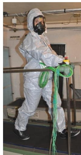
Figure 2: Test of physiologic response in climatic chamber
