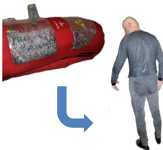
Figure 5: Rapid increase of moisture up to 100 % rel. hum. caused that the proband was all wet after 20 minutes.
